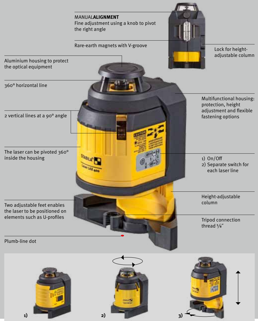
1) Park position. 2) Housing can pivot 360° inside the U-shaped housing. 3) The height of the laser can be adjusted thanks to the extendable column. The two adjustable feet enables the laser to be positioned on elements such as U-profiles.
